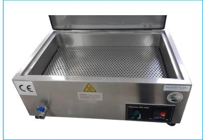
With cover, stainless steel, for heating Pedilon® sheets, with thermostat controlled heater and safety thermostat. Designed for Prosthetic Orthoses workshops top cover, cover opening handle available
