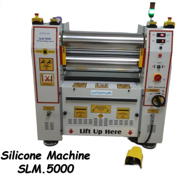
For mixing larger quantities of silicone [up to 3 kg], rolling them into large silicone sheets with thicknesses ranging from 0.1 to 35 mm and sizes up to max.650 mm, manual processing of highly viscous HTV silicones.
